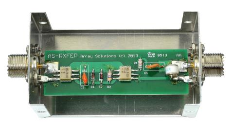
**Figure 3** — View of unit with snap-on cover removed. The miniature gas discharge tube at the antenna input is clearly visible on the right side.
